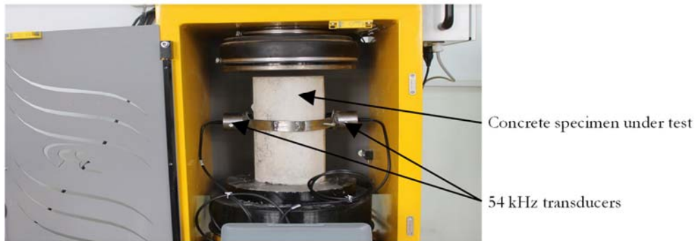
Figure 5: Experimental procedure for compressive tests.
