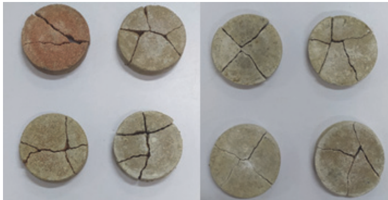
Figure 11: Representation of the cracked stones from the triaxial experiments.
