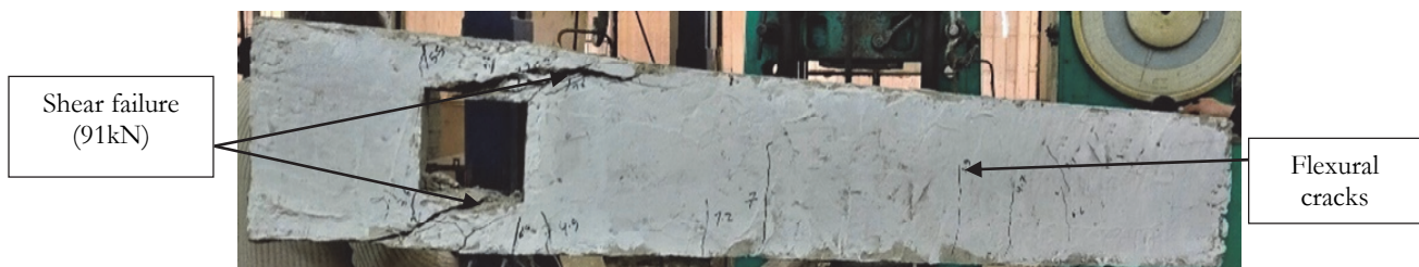
Figure 26: Failure mode for (B3S)
