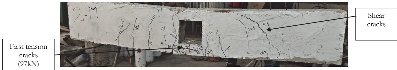
Figure 21: Failure mode for (B2M)
