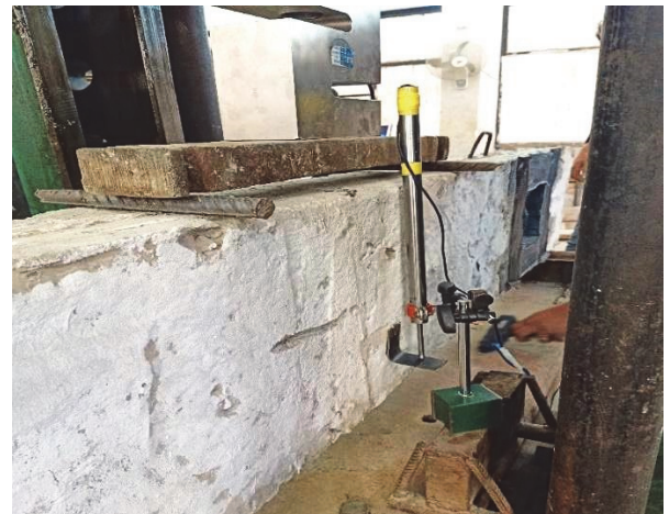
Figure 7: Deflection measurement by LVDT
