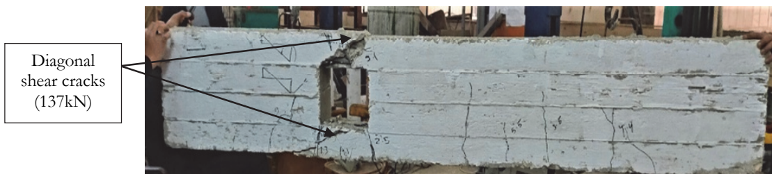
Figure 25: Failure mode for (B3L)
