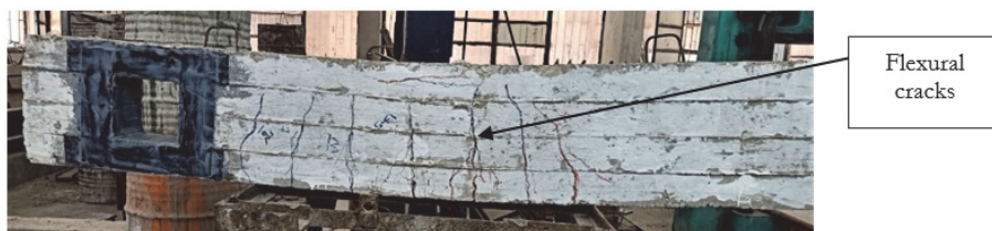
Figure 29: Failure mode for (B4S)
