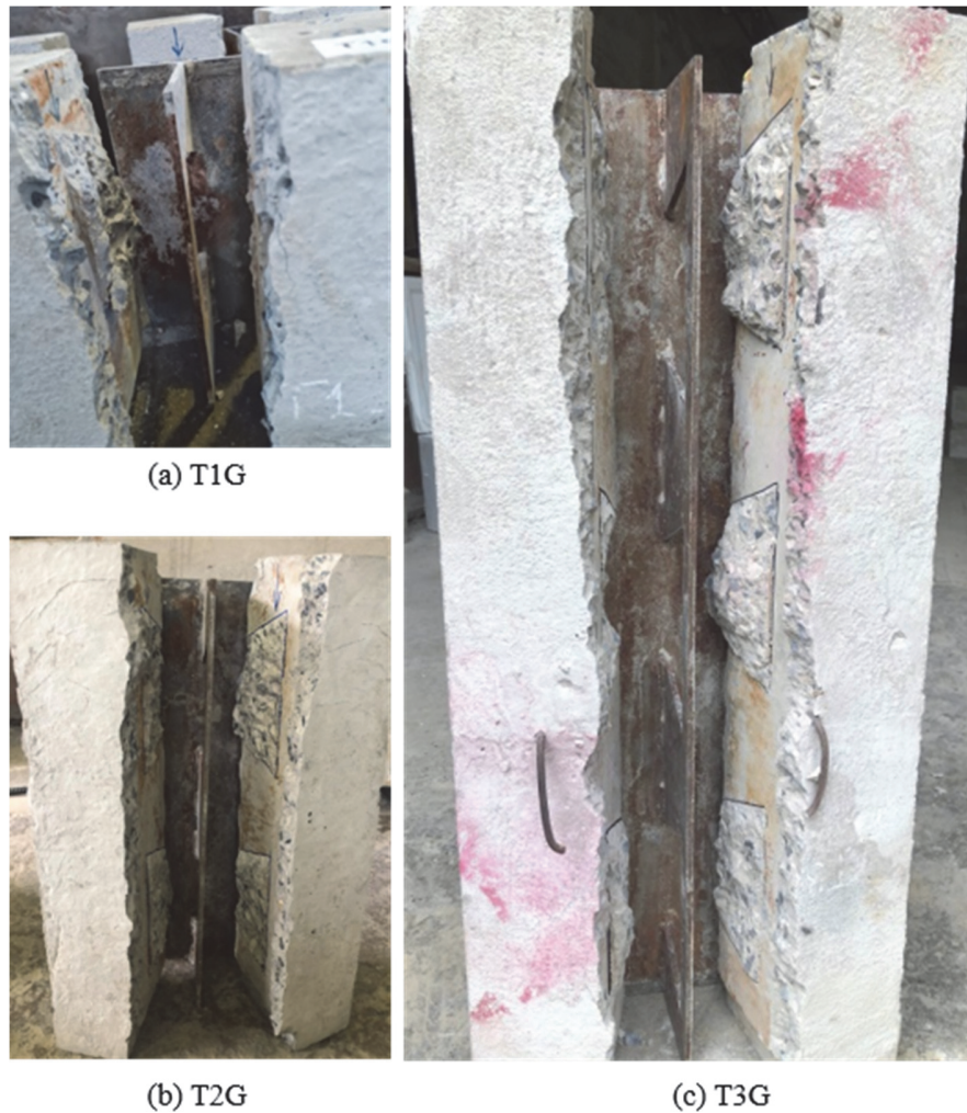
Figure 7: Failure of specimens.
