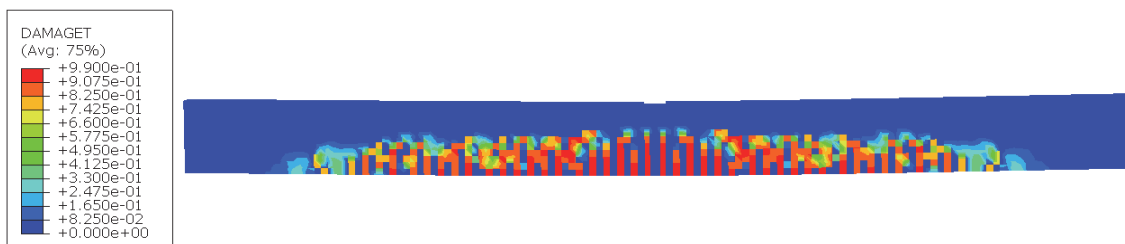
Figure 9: Cracking pattern in simulation.
