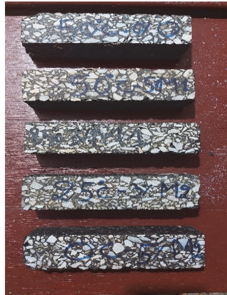
Figure 4: Prismatic test piece (200×50×50 mm).
