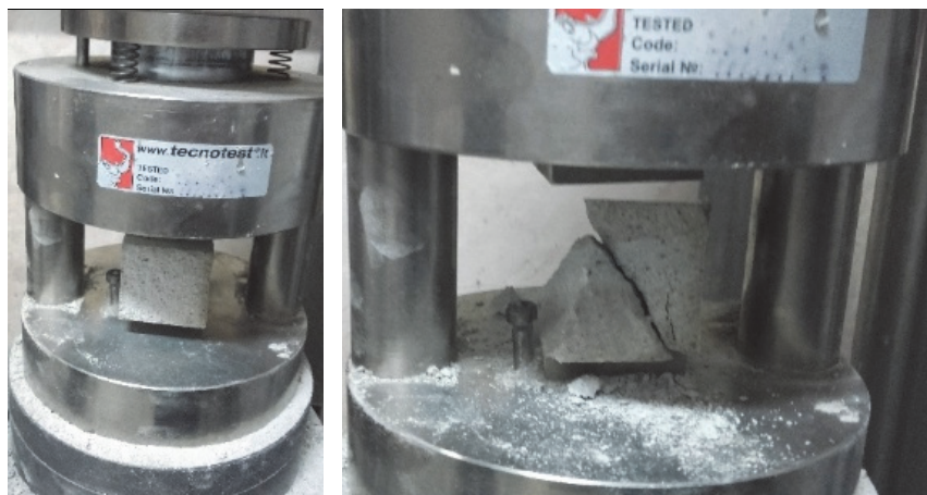
Figure 1: Compression strength test.
