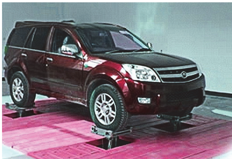
Figure 9: The employed Servotest four-poster testing facility.
