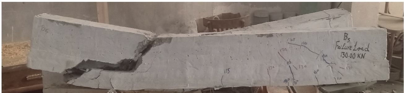
Figure 19: Concrete crack patterns at ECC beam (B 05).
