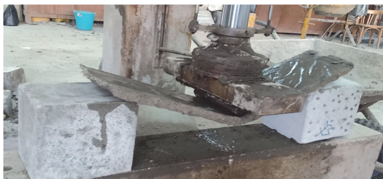
Figure 1: Response of ECC under Flexural Loading.
