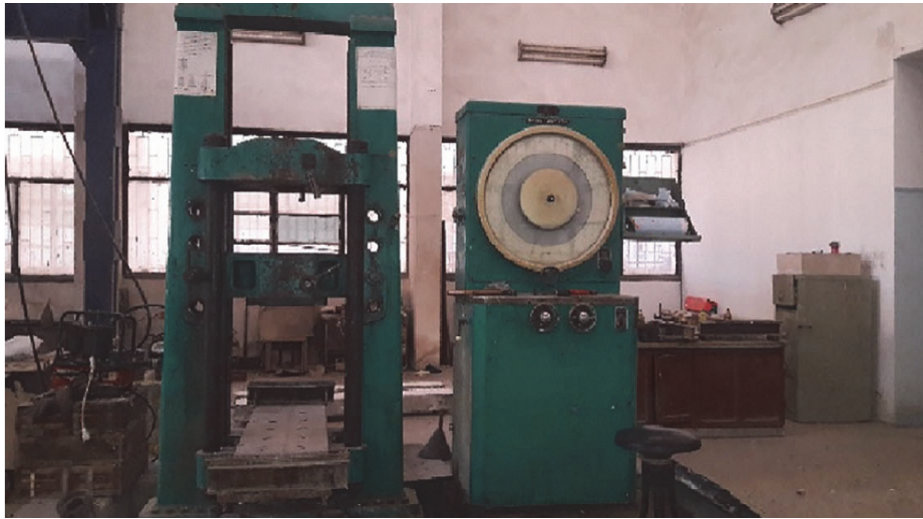
Figure 2: MTS machine, with Capacity 1000KN.
