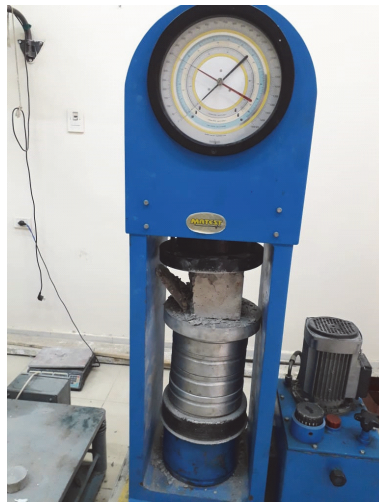
Figure 3: Standard compression test for cube specimens.
