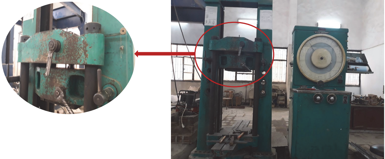
Figure 4: Standard tension test for steel reinforcement.
