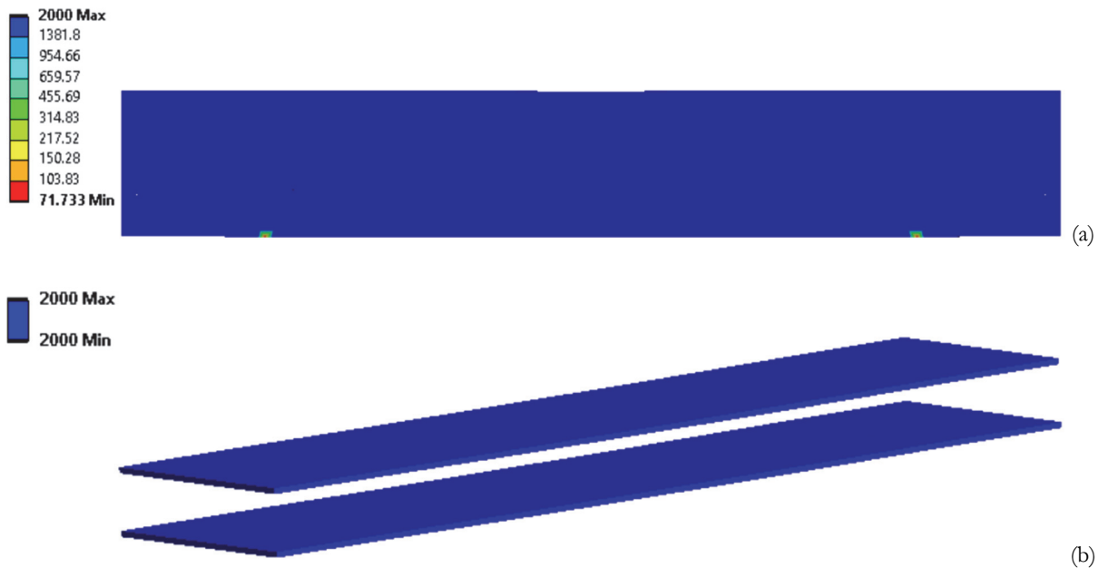
Figure 13: Fatigue life distribution modelled using finite element to determine the critical region based on; (a) front view of sandwich panel geometrical body, (b) bonding area for SP-2 at \sigma_{min} = -0.2 with a load of 37422N
