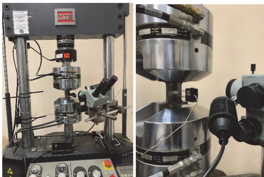
Figure 3: Test equipment for SCT specimens fatigue crack growth tests.
