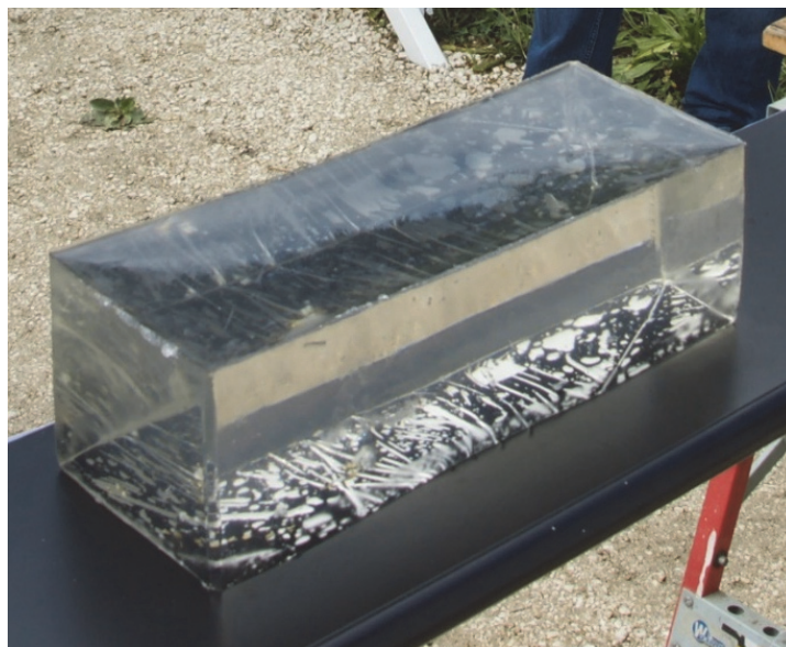
Figure 3: Baligel block showing its transparency and clarity.
