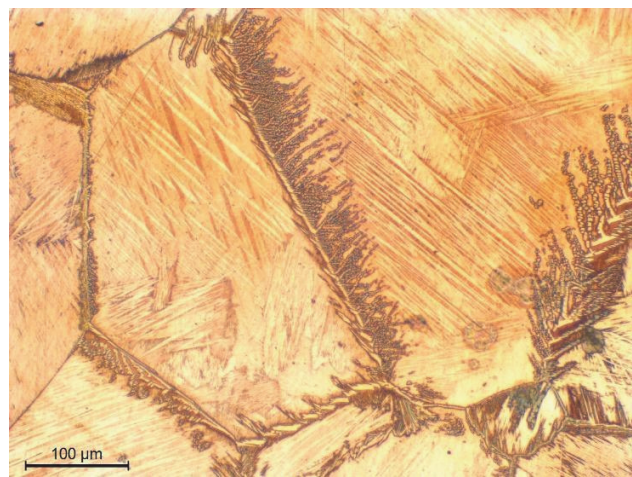
Figure 2b: Alloy microstructure after ferric chloride metallographic etch coarse-equi-oriented needle microstructure.
