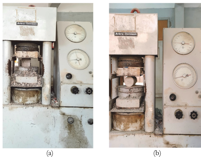
Figure 6: Test setup (a) Compression test (b) Splitting tensile test.
