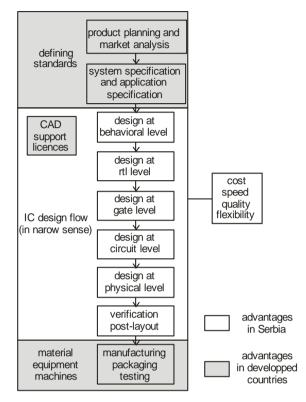
Fig. 2 IC design flow
