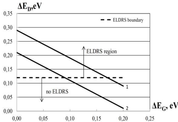
**Fig. 7** The effect of bandgap narrowing  $\Delta E_G$  on the excited energy  $\Delta E_D$ . The dotted line presents the boundary between ELDRS region and region where ELDRS is absent (ELDRS-free).
