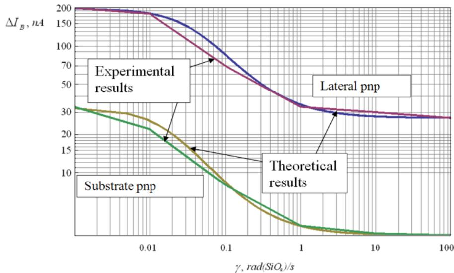
**Fig. 4** Excess base current versus dose rate. Experimental [18] and calculated data from relationship (11).
