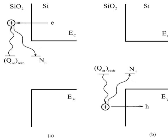
**Fig. 2** Conversion of oxide charge  $(Q_{ot})_{rech}$  to interface trap  $N_{it}$ : capture of an electron  $e$  (a), emission of a hole  $h$  (b).  $E_c$  and  $E_v$  are energy levels of Si conduction and valence band
