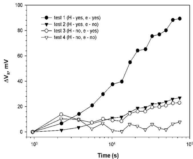
**Fig.1** Interface-trap component of the threshold voltage shift  $\Delta V_{it}$  versus the annealing time in the hydrogen atmosphere (After Ref. [5])
