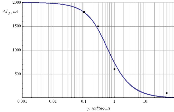
**Fig. 5** Excess input base current LM158 versus dose rate. Experimental [19] (dots) and calculated data from conversion model (11).
