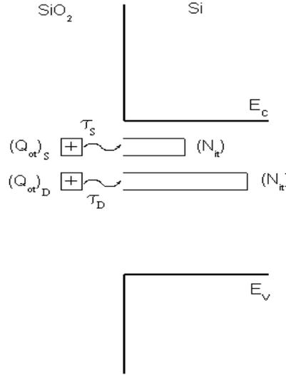
**Fig. 3** The shallow  $(Q_{ox})_S$  and deep  $(Q_{ox})_D$  oxide trapped charges with conversion time  $\tau_S$  and  $\tau_D$
