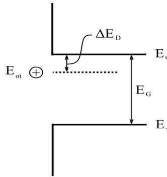
**Fig. 6** The energy of thermal excitation  $\Delta E_D$  from level of positive trap in the oxide  $E_{ot}$  to conduction band edge  $E_c$ .  $E_G$  is bandgap of semiconductor.
