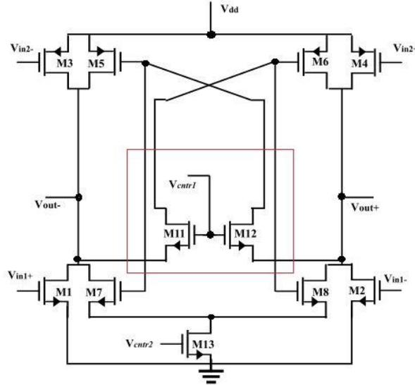
**Fig. 4** Delay Cell due to high  $V_{ctr2}$
