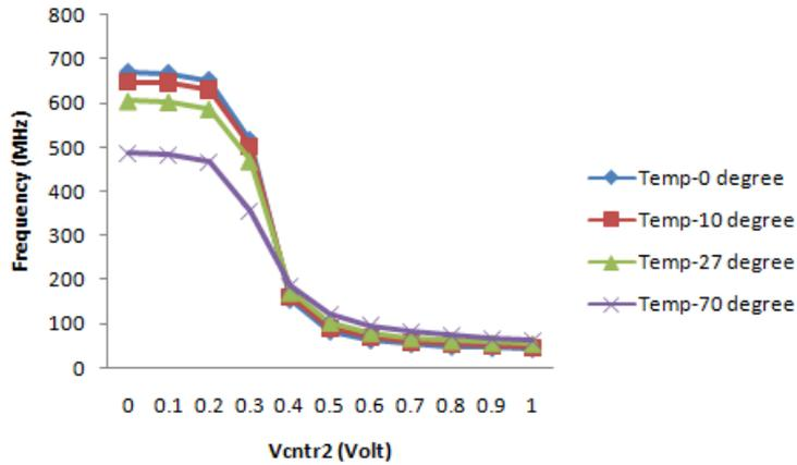
Fig. 5 Tuning range of VCO at different temperatures for  $V_{cntr1}=0.2V$  and  $V_{cntr2}$  varies from 0V to 1V (Pre layout simulation)
