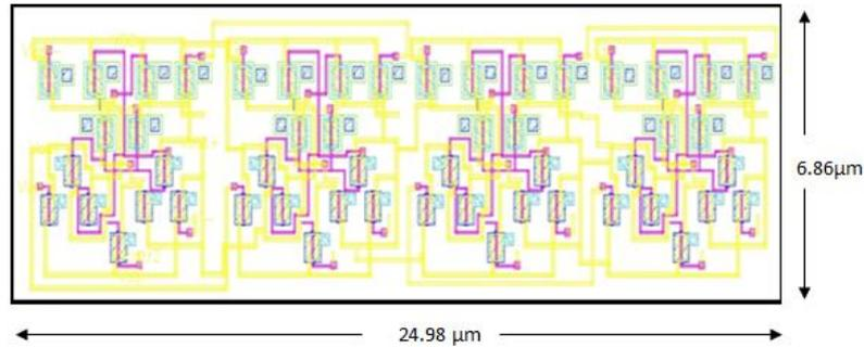
**Fig. 10** Layout of the 4 stage VCO
