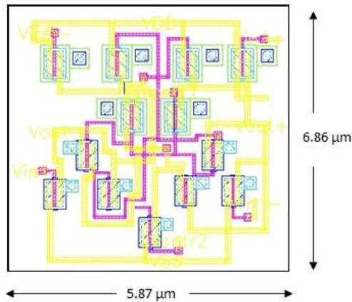
**Fig. 9** Layout of the proposed delay cell
