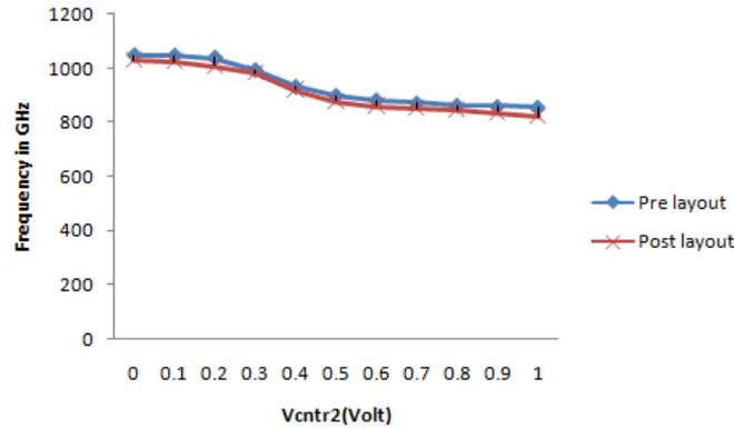
**Fig. 8** Tuning range of VCO at normal temperature for  $V_{cntr1}=0.77\text{V}$  and  $V_{cntr2}$  varies from  $0\text{V}$  to  $1\text{V}$  (Pre and post layout simulation at  $27^\circ$ )
