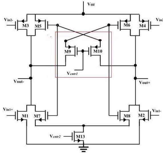
**Fig. 3** Delay circuit for low voltage of  $V_{ctr1}$
