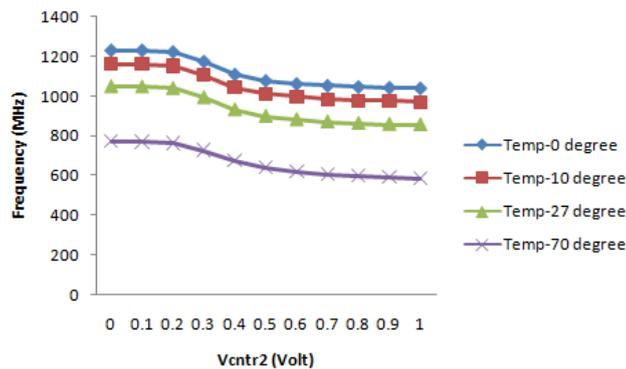
**Fig. 7** Tuning range of VCO at different temperatures for  $V_{ctr1}=0.77$  V and  $V_{ctr2}$  vary from 0V to 1V.
