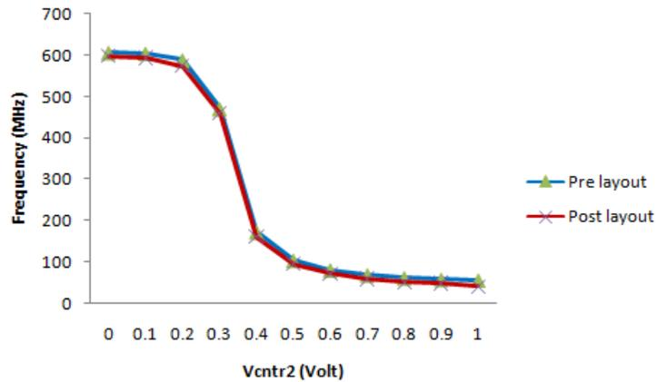
Fig. 6 Tuning range of VCO at normal temperature for  $V_{cntr1}=0.2V$  and  $V_{cntr2}$  varies from 0V to 1V (Pre and post layout simulation at 27°)
