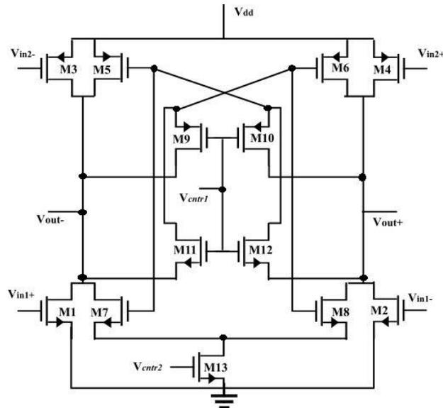
Fig. 1 Delay Cell
