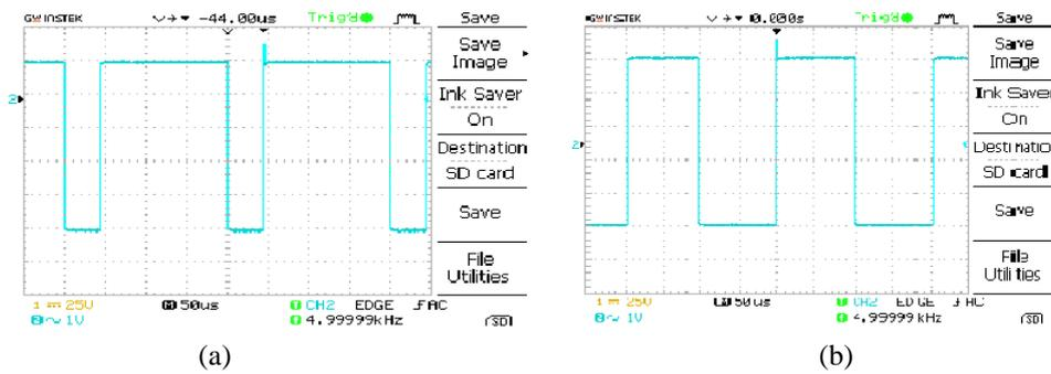
**Fig. 15** PWM Signal fed to the Buck converter at (a) 75% duty cycle, (b) 50% duty cycle
