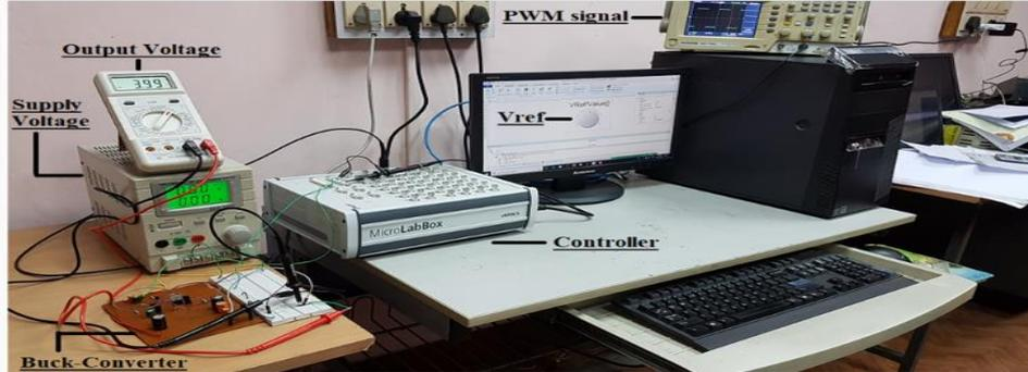
**Fig. 12** Complete hardware setup with 4 volts as reference
