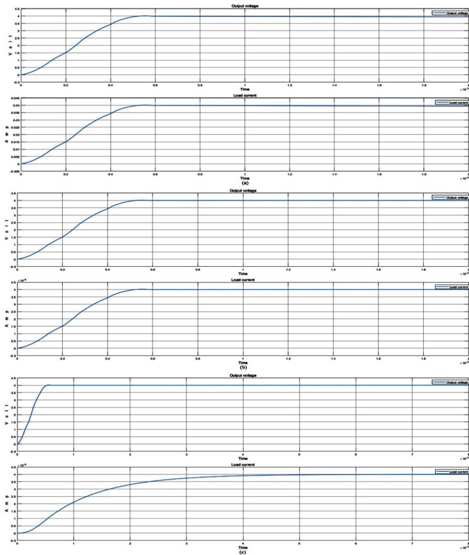
**Fig. 11** Simulation of the system under different load conditions. (a) with 100  $\Omega$  resistance, (b) with 100 k $\Omega$  resistance, (c) with R-L load consisting of 100 k $\Omega$  resistance and 100 H inductor
