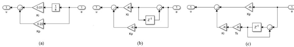
**Fig. 4** (a) PI Controller in the continuous domain, (b) PI Controller in the discrete Z domain, (c) PI Controller in the discrete  $\delta$  domain
