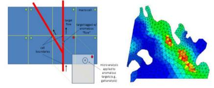
Fig. 11 Two partition strategies: (a) Euler formation of a transportation network; (b) Lagrange formulation of a lake.
