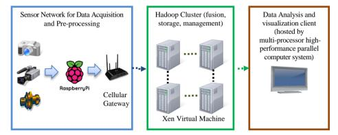
Fig. 1 Hardware Configuration of SOIS-Hadoop (dash-line indicates those internet link).
