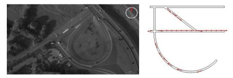
**Fig. 10** (a) traffic status acquired using UAV-mounted optical-electro sensor array; (b) expected traffic flow derived from empirical data and Equation (6).
