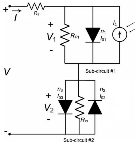
**Fig. 10** An improved solar cell dc lumped-parameter equivalent circuit model, proposed by P. J. Roland et al [50] as a further improvement to the models proposed by Araujo de Castro et al [41] and by García-Sánchez et al [48]. The series resistor has been restored as a necessary element to describe the parasitic series resistance.
