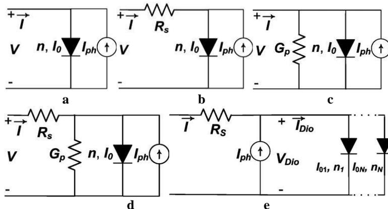
**Fig. 1** Typical generic solar cell dc lumped-parameter equivalent circuit models showing the photo-generated current source with: (a) a single ideal diode in parallel; (b) plus a series resistance; (c) plus a parallel conductance; (d) plus both series resistance and parallel conductance; and (e) several ideal diodes plus a series resistance.
