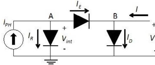
**Fig. 2** DC lumped-parameter equivalent circuit model proposed by Mazhari [38] to describe the illuminated  $I$ - $V$  characteristics of organic solar cells considering a non-constant photo-generated current.
