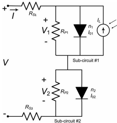
**Fig. 8** Organic solar cell dc lumped-parameter equivalent circuit model proposed by Zuo et al [36] to describe the S-shaped kink. It includes the conventional single ideal diode with series and shunt resistances (sub-circuit #1), and series-connected sub-circuit #2 with a single Schottky diode and a parallel resistor, and additional series resistor.
