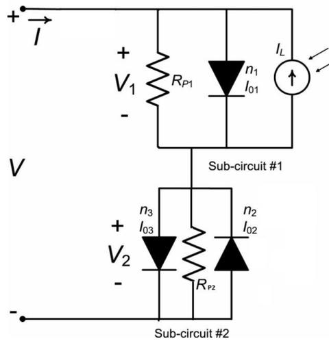
**Fig. 9** Second solar cell dc lumped-parameter equivalent circuit model, proposed as an improvement by Araujo de Castro et al [41]. It is said to improve on the previous equivalent circuit model by García-Sánchez et al [48]. The previously present series resistor has been eliminated. The previously eliminated shunt resistor  $R_{P2}$  has been added again in parallel, but now with the two diodes in the series-connected sub-circuit #2
