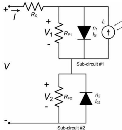
**Fig. 3** Solar cell dc lumped-parameter equivalent circuit model proposed by Araujo de Castro et al [10] to describe the S-shaped kink. It includes a conventional single ideal diode with series and shunt resistances (sub-circuit #1) and series-connected sub-circuit #2 consisting of a single ideal diode and a parallel resistor to model the S-shaped kink
