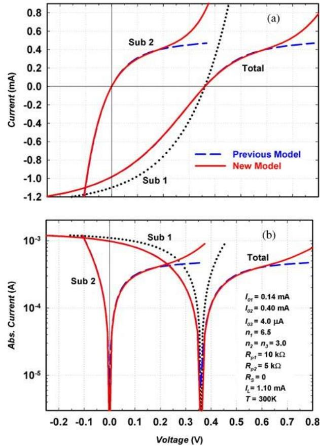
**Fig. 6** Comparison of the S-shaped kinks in two synthetic illuminated  $I$ - $V$  characteristics, presented in linear (a) and semi-logarithmic (b) scales, as generated by the dc lumped-parameter equivalent circuit models shown in Figs. 3 and 5, using the parameter values indicated within the lower pane (dotted black lines = sub-circuit #1, dashed blue lines = first model by Araujo de Castro et al [10], continuous red lines = model by García-Sánchez et al [48]).
