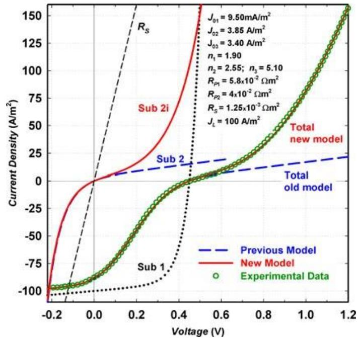
**Fig. 7** Illuminated  $I$ - $V$  characteristics of an experimental organic solar with S-shaped kink (dashed black straight line = Series Resistance  $I$ - $V$  curve, dotted black line = sub-circuit #1  $I$ - $V$  curve, continuous dashed blue lines = sub-circuit #2  $I$ - $V$  curve and total model playback of previous model, red lines = sub-circuit #2i  $I$ - $V$  curve and total model playback of newer model, green circles = measured  $I$ - $V$  data).
