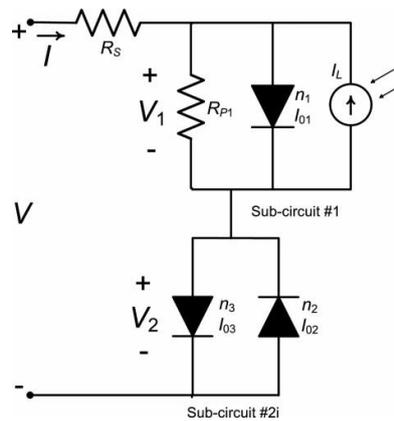
**Fig. 5** The solar cell dc lumped-parameter equivalent circuit model proposed by García-Sánchez et al [48] to allow describing the S-shaped kink. It includes the same conventional single ideal diode with series and shunt resistances as before (sub-circuit #1), but the series-connected sub-circuit #2 has been modified to replace the previous resistor  $R_{p2}$  by a third diode connected with reversed polarity, the same as that of the diode of sub-circuit #1.
