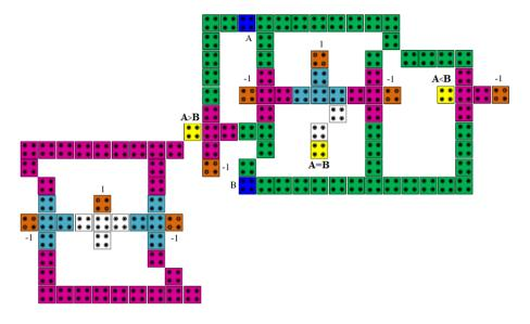
Fig. 4. The utilized QCA comparator circuit in [11]
