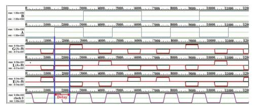
Fig. 10. The results for the designed 1-bit comparator circuit
