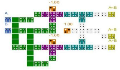
Fig. 6. The utilized QCA comparator circuit in [16]
