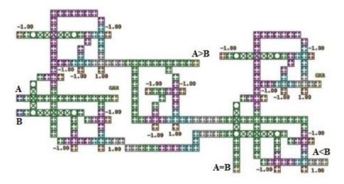
Fig. 3. The utilized QCA comparator circuit in [10]
