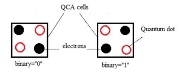
Fig. 1. The possible stats for the QCA cell [5]
