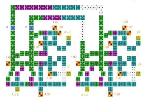
Fig. 7. The utilized QCA comparator circuit in [17] This QCA comparator circuit requires 0.23  $\mu$ m<sup>2</sup> area and 220 QCA cells.
