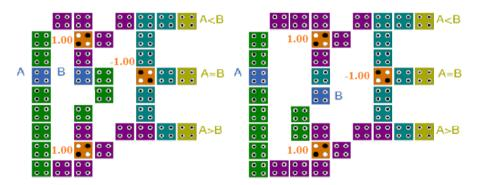
Fig. 5. The utilized QCA comparator circuits in [12]
