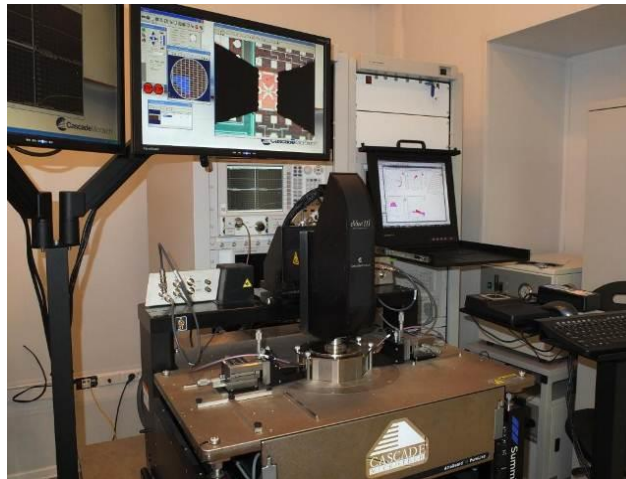
Fig.7 Specialized microwave test system
