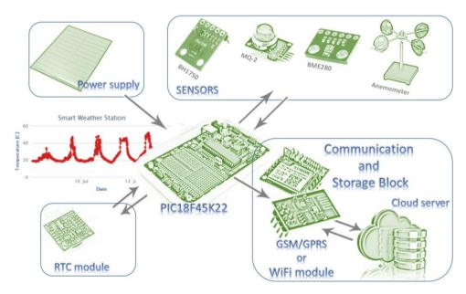
**Fig. 2** Block scheme of the smart weather station. Block scheme is based on [6]. The measured results for temperature are given as an example.
