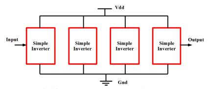
Fig. 13 General approach for a chain of 4 Inverters
