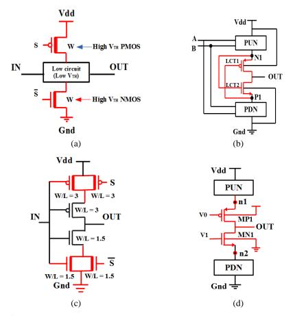
Fig. 1 Leakage power approaches (a) MTCMOS [21] (b) LECTOR [22] (c) Sleepy Stack [23] (d) INDEP [24]
