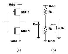
Fig. 9 (a) Inverter Circuit schematic (b) RC equivalent circuit
