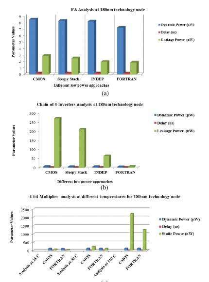
Fig. 14 Comparison of proposed FORTRAN approach with reported approaches, (a) & (b) comparison with different approaches and (c) comparison at different temperature ranges
