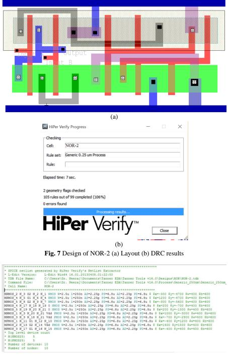
Fig. 8 Netlist extract on the physical layout of NOR-2 cell.
