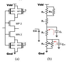
Fig. 11 (a) Sleepy Stack Inverter Circuit schematic (b) RC equivalent circuit
