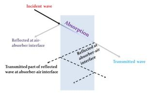
Fig. 1 Schematic representation of absorbing type EMI shielding mechanism
