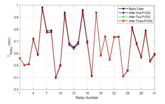
Fig. 6 Overcurrent relay operation time for all cases studied.
