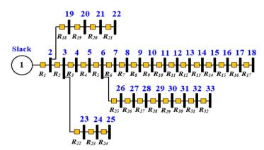
Fig. 1 Single diagram of test system IEEE 33-bus RDN.
