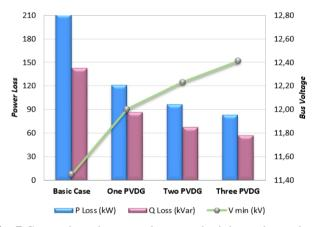
Fig. 7 Comparison the power losses and minimum bus voltage.
