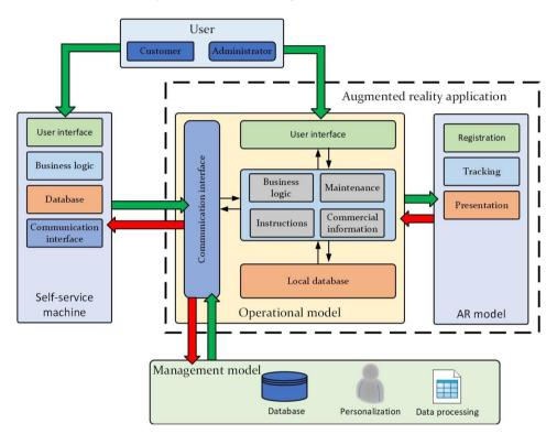
Fig. 13 Smart-shop kiosk architecture based on augmented reality
