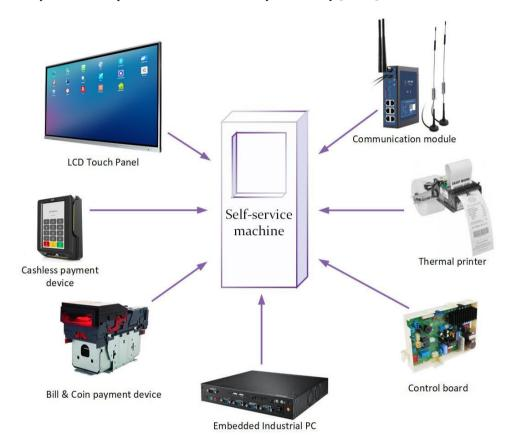
Fig. 5 Components of a typical self-service automated system
