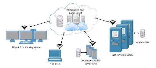
Fig. 10 Architecture of the smart-shop network system
