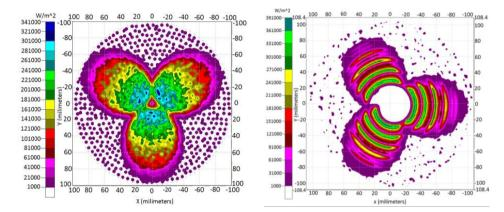
Fig. 11 Solar flux distribution on the absorber Fig. 12 Solar flux distribution on the absorber surface - 119 401 simulated rays
