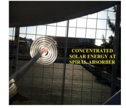
Fig. 1 Experimental model of a parabolic offset solar concentrator system
