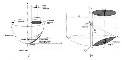
Fig. 5 a) Section of the offset parabolic solar dish concentrator from baseline paraboloid; b) Process of determining a offset parabolic solar dish concentrator
