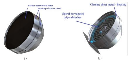
Fig. 7 Two types of solar thermal receivers: a) flat plate painted black; b) spiral pipe
