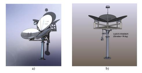
Fig. 4 a) Working position of the offset parabolic dish solar concentrator (axonometric view); b) safety position (elevation angle of 900)
