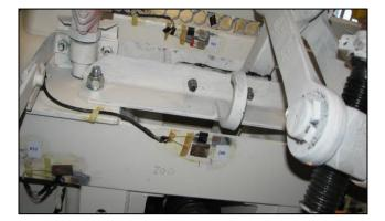
Fig. 8 Strain gauge no. 2 - placement on wagon prototype during test
