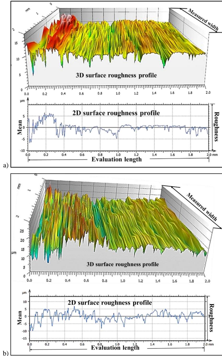
**Fig. 5** 2D profiles and 3D topographies for surface roughness of (a) best quality ratchet gear, (b) poor quality ratchet gear
