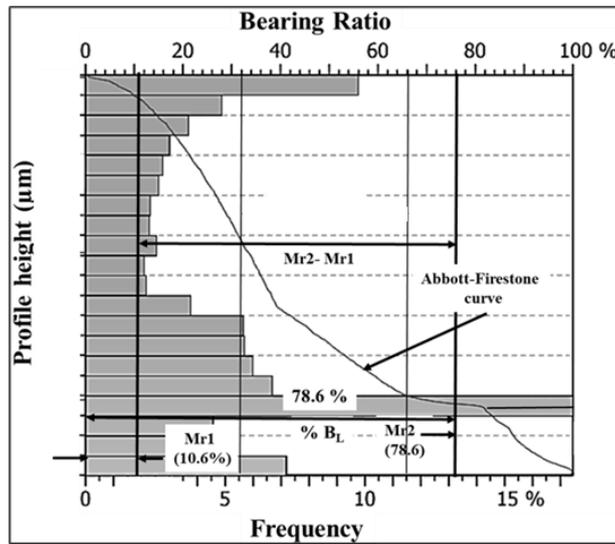
Fig. 8 Bearing area curve for poor surface quality ratchet gear
