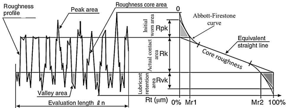
Fig. 6 Theoretical concept of bearing area curve
