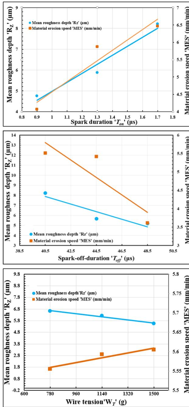
**Fig. 3** Effect of wire-EDM parameters on mean roughness depth and material erosion speed during manufacturing of ratchet gear: a) Effect of spark duration; b) Effect of spark-off duration; c) Effect of wire tension
