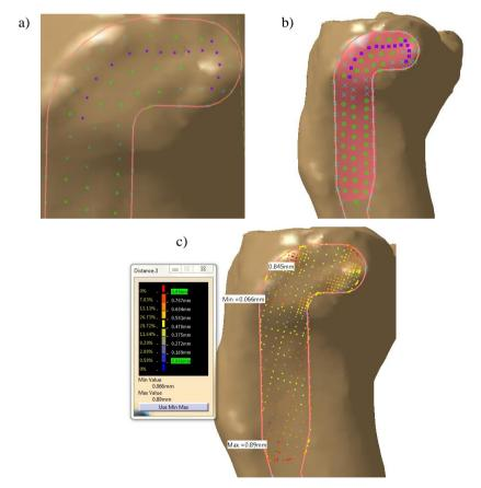
Fig. 6 Definition of MIF-LTP contact surface with additional parametric points:a) Additional points (square);b) New surface model with added points;c) Deviation analysis between input and newly created surface models
