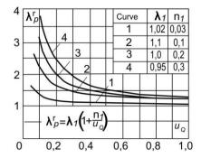
Fig. 2 Characteristics of excess air ratio depending on a wide range of boiler load [11]
