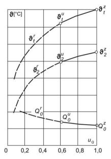
**Fig. 4** Dependence of theoretical combustion temperature  $(\mathcal{G}_i)$ ; temperature of combustion products that leave the combustion chamber  $(\mathcal{G}_2)$ ; and heat that is received by the screens of the combustion chamber  $(\mathcal{Q}_0)$  of boiler load with coal powder combustion OP-230, OP-650k, BP-1150 and BB-1150 [11].
