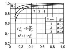
Fig. 1 Combustion chamber efficiency depending on a wide range of boiler load [11]
