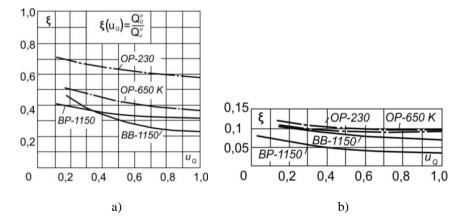
**Fig. 3** Dependence of the relative heating of the combustion chamber walls (a) and flue pipes, or economizer (b) of the boiler load with coal powder combustion OP-230, OP-650k, BP-1150 and BB-1150 [11]
