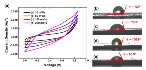
**Fig. 6** (a) Cyclic voltammetry (CV) curves for the AgNW coated CNT/PEDOT:PSS/PDMS composite at different scan rates. (b-e) Optical images of water drop shape on (b) pure PDMS, (c) PEDOT:PSS/PDMS, (d) CNT/PEDOT:PSS/PDMS, and (e) AgNW coated CNT/PEDOT:PSS/PDMS.
