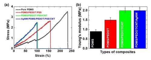
**Fig. 4** (a) Stress-strain curves and (b) Young's modulus of PDMS composites using different types of functional fillers.
