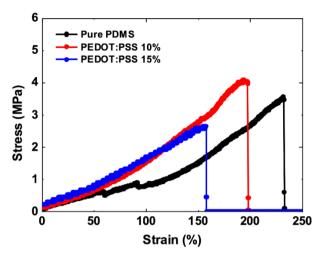
Fig. 2 Stress-strain curves of PDMS composites with the different PEDOT:PSS contents.
