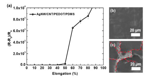
**Fig. 5** (a) Normalized resistance change of the AgNW-coated CNT/PEDOT:PSS/PDMS composites as a function of tensile strain values. Top-view SEM images of the AgNW-coated CNT/PEDOT:PSS/PDMS composites under the tensile strain of (b) 40% and (c) 60%.
