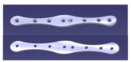
Fig. 13 Final model of customized plate
