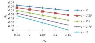
Fig. 2 Variation of load carrying capacity with respect to  $H_m$  and  $\gamma$
