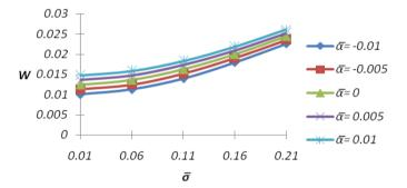
Fig. 12 Variation of load carrying capacity with respect to  $\overline{\sigma}$  and  $\overline{\alpha}$
