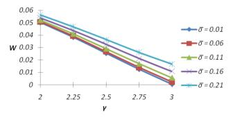
Fig. 7 Variation of load carrying capacity with respect to  $\gamma$  and  $\overline{\sigma}$
