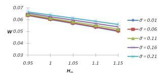
Fig. 3 Variation of load carrying capacity with respect to  $H_m$  and  $\overline{\sigma}$
