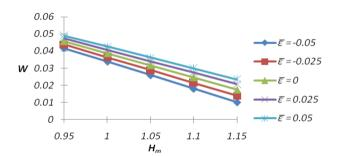
**Fig. 4** Variation of load carrying capacity with respect to  $H_m$  and  $\bar{\varepsilon}$
