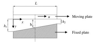
Fig. 1 Configuration of the bearing system
