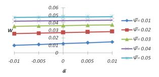
**Fig. 17** Variation of load carrying capacity with respect to  $\overline{\alpha}$  and  $\overline{\psi}$
