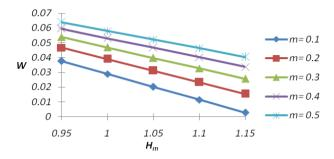
Fig. 6 Variation of load carrying capacity with respect to  $H_m$  and m
