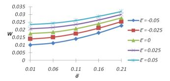
**Fig. 11** Variation of load carrying capacity with respect to  $\overline{\sigma}$  and  $\overline{\varepsilon}$
