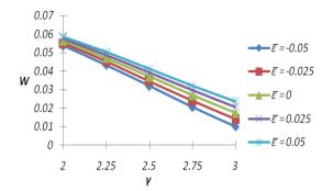
**Fig. 8** Variation of load carrying capacity with respect to  $\gamma$  and  $\bar{\varepsilon}$
