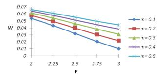
Fig. 10 Variation of load carrying capacity with respect to  $\gamma$  and m
