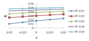
Fig. 16 Variation of load carrying capacity with respect to  $\overline{\varepsilon}$  and  $\overline{\psi}$
