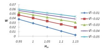
**Fig. 5** Variation of load carrying capacity with respect to  $H_m$  and  $\overline{\psi}$
