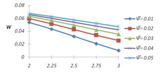
Fig. 9 Variation of load carrying capacity with respect to  $\gamma$  and  $\overline{\psi}$
