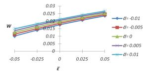
Fig. 15 Variation of load carrying capacity with respect to  $\bar{\varepsilon}$  and  $\bar{\alpha}$
