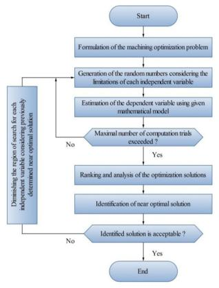
Fig. 1 Monte Carlo method flowchart for solving machining optimization problems
