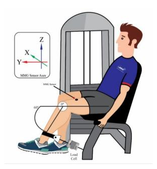
**Fig. 1** Scheme of the experimental setup. The MMG sensor (triaxial accelerometer) was placed over the *rectus femoris* muscle belly and knee angle was positioned in 60° of flexion with a load cell
