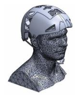
Fig. 4 Virtual model of 3D scanned head and designed bicycle helmet
