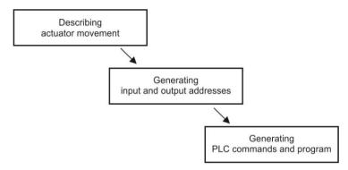
Fig. 4 Block scheme of automatic PLC programming of the sequential control of pneumatic actuators
