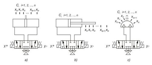
Fig. 2 Pneumatic system with more than two end positions with: a) Symmetric actuator, b) Asymmetric actuator, c) Semi-rotary drive
