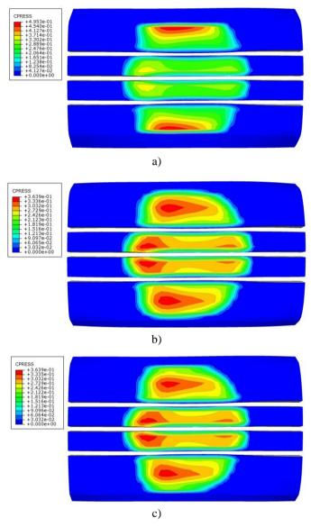
Fig. 7 Tire footprint shapes at full braking for a)  $R_1$ =53.8mm, b)  $R_1$ =64.4mm and c)  $R_1$ =75.0mm
