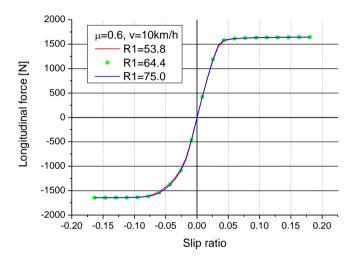
Fig. 6 The effect of sidewall radius variation on full-breaking-to-full-acceleration curve
