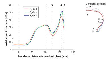
**Fig. 3** Carcass stress comparison for tire variations that differ by value of R<sub>1</sub>. The characteristic points on carcass are: 1 – midpoint, 2 – point closest to the end of returning portion, 3 – point on the edge of filler, 4 – point on the upper edge or bead wire and 5 – point on the lower edge or bead wire
