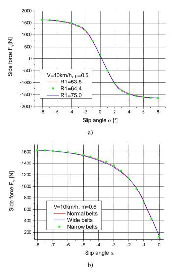
Fig. 8 Cornering curves for models with three different values of a) sidewall radius and b) belt width
