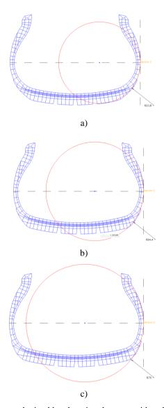
**Fig. 2** Three tire instances obtained by changing the upper sidewall radius  $(R_1)$ : a)  $R_1$ =53.8mm, b)  $R_1$ =64.4mm and c)  $R_1$ =75.0mm. The change affects the sharpness of shoulder area and the width of the crown (without affecting the belt width)
