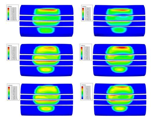
**Fig. 9** Tire footprint shapes; first row:  $R_1$ =53.8 mm, second row:  $R_1$ =64.4 mm, third row:  $R_1$ =75.0 mm. Left column corresponds to cornering at 2 degrees and right column to cornering at 4 degrees
