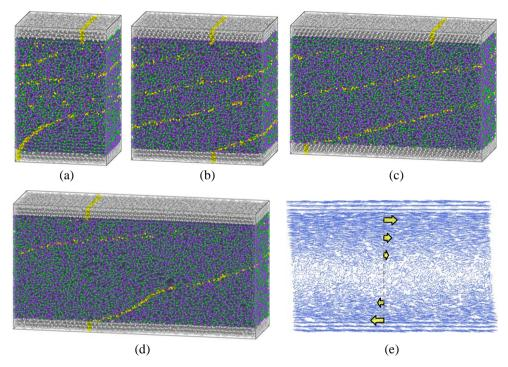
**Fig. 3** Structures of the central fragment of different silica specimens after 1 ns of sliding: (a)  $L_x = 10.0$  nm, T = 400 K; (b)  $L_x = 15.0$  nm, T = 600 K; (c)  $L_x = 22.5$  nm, T = 600 K; (d)  $L_x = 30.0$  nm, T = 600 K. (e) Trajectories of atoms of the specimen with  $L_x = 15.0$  nm after 2.0 ns of sliding at 700 K Arrows show the velocity distribution of atoms
