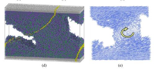
**Fig. 2** Structures of the central fragment of different silica specimens after 1 ns of sliding: (a)  $L_x = 10.0$  nm, T = 300 K; (b)  $L_x = 15.0$  nm, T = 500 K; (c)  $L_x = 22.5$  nm, T = 500 K; (d)  $L_x = 30.0$  nm, T = 500 K. (e) Trajectories of atoms of the specimen with  $L_x = 15.0$  nm after 1.0 ns of sliding at 500 K. Arrow marks the direction of atoms rotation
