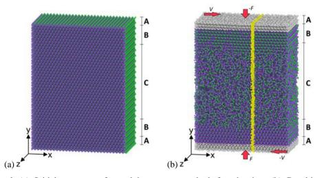
Fig. 1 (a) Initial structure of an alpha-quartz sample before heating. (b) Resulting structure of the amorphous silica sample and a loading scheme for sliding simulation. Hereafter the atoms colored in yellow are used to indicate the features of deformation along the sample. The following zones are indicated: A – atoms under loading (loaded layers), B – crystallite layers, C – melted/amorphous area. Purple color denotes O atoms, green – Si atoms
