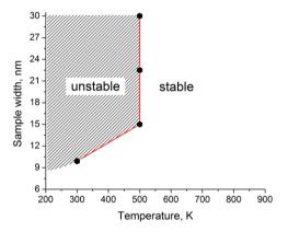
Fig. 4 Dependence of critical conditions for transitions of sliding regime on sample width and temperature conditions
