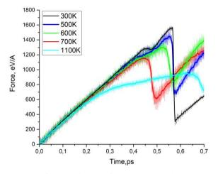
Fig. 5 Time dependence of the resistance force to tangential motion within the silica amorphous interlayer in the base sample at various thermal conditions
