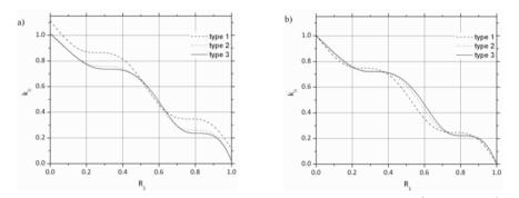
**Fig. 7** Variation of CLP with  $R_1$  for cl-cl beam and  $\theta_2 = 0.8$ : a)  $\delta = \frac{1}{20}$ , b)  $\delta = \frac{1}{100}$
