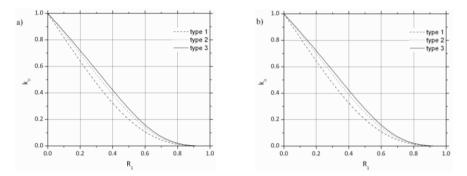
**Fig. 10** Variation of CLP with  $R_1$  for cl-fr beam and  $\theta_2 = 0.8$ : a)  $\delta = \frac{1}{20}$ , b)  $\delta = \frac{1}{100}$
