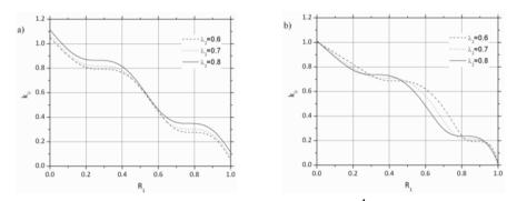
**Fig. 8** Variation of CLP with  $R_1$  for cl-cl beam and  $\delta = \frac{1}{20}$ : a) type 1, b) type 3
