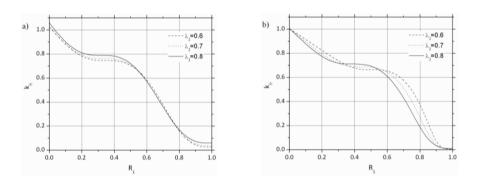
**Fig. 14** Variation of CLP with  $R_1$  for cl-pn beam and  $\delta = \frac{1}{20}$ : a) type 1, b) type 3
