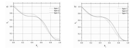
**Fig. 13** Variation of CLP with  $R_1$  for cl-pn beam and  $\theta_2 = 0.8$ : a)  $\delta = \frac{1}{20}$ , b)  $\delta = \frac{1}{100}$
