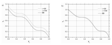
**Fig. 9** Variation of CLP with  $R_1$  for cl-cl beam and  $\theta_2 = 0.8$ : a) type 1, b) type 3
