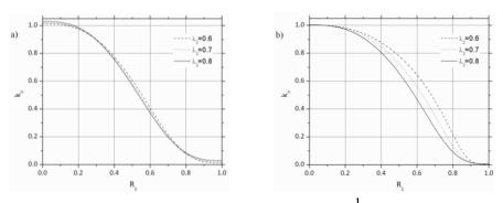
**Fig 5** Variation of CLP with  $R_1$  for pn-pn beam and  $\delta = \frac{1}{20}$ : a) type 1, b) type 3
