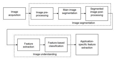
Fig. 1 Computer vision block diagram
