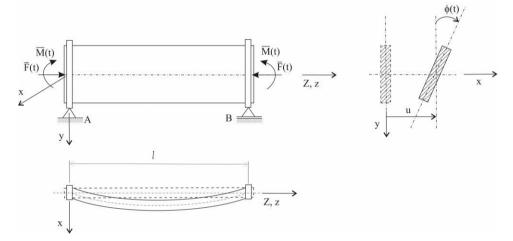
Fig. 1 Geometry of a thin-walled beam system
