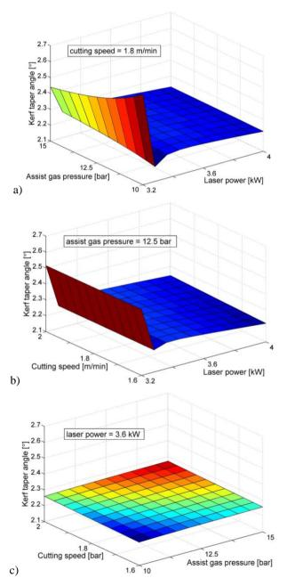
**Fig. 2** Change of kerf taper angle with respect to: a) interaction effect of laser power and assist gas pressure, b) interaction effect of laser power and cutting speed, c) interaction effect of cutting speed and assist gas pressure
