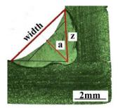
**Fig. 5** The methodology of weld geometry measurements
