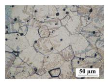
Fig. 1 The microscopic view of X2CrTiNb18 (AISI 441) steel
