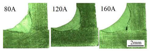
Fig. 6 Effect of welding current on the weld geometry – specimens from group E
