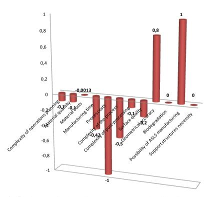
**Fig. 5** *Values* (*V*) of variables for determining the applicability of EBM in ASLS manufacturing
