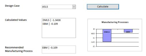
Fig. 8 Result of the Calculator for the assessment of selected AMP applicability for ASLS manufacturing
