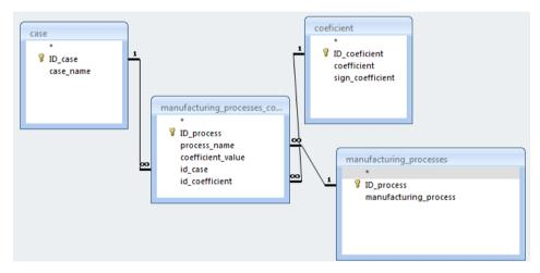
Fig.7 Relational database schema of Calculator
