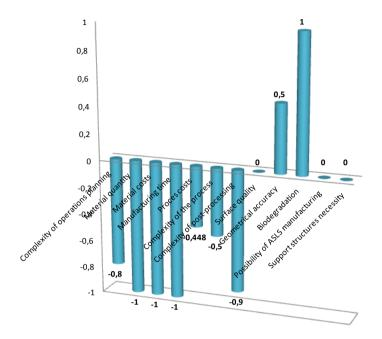
**Fig. 3** *Values* (*V*) of variables for determining the applicability of 3D bioplotter in ASLS manufacturing
