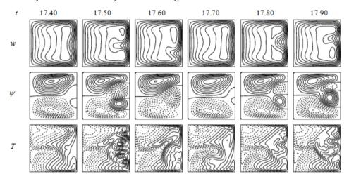
Fig. 12 Velocity contour (top & middle) and isotherm (bottom) for Tr = -30
