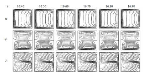
Fig. 18 Velocity contour (top and middle) and isotherm (bottom) for Tr = -1100
