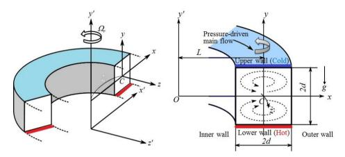
Fig. 1 (a) Physical domain (b) Cross-section of the system
