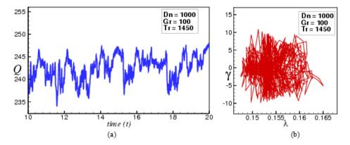
Fig. 9 Transient solution for Tr = 1450 (a) Q as a function of time, (b) PS of (a)
