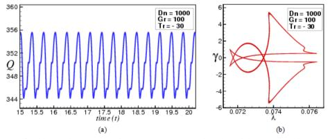
Fig. 11 Transient solution for Tr = -30 (a) Q as a function of time, (b) PS of (a)
