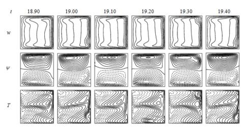
Fig. 10 Velocity contour (top & middle) and isotherm (bottom) for Tr = 1450
