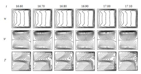
Fig. 8 Velocity contour (top & middle) and isotherm (bottom) for Tr = 1300
