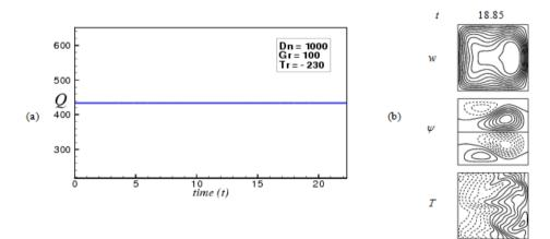
Fig. 13 Transient solution for Try = -230 (a) Q as a function of time, (b) Velocity contour (top & middle) and isotherm (bottom) for Try = -230
