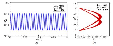
Fig. 17 Transient solution for Tr = -1100 (a) Q as a function of time (b) PS of (a)
