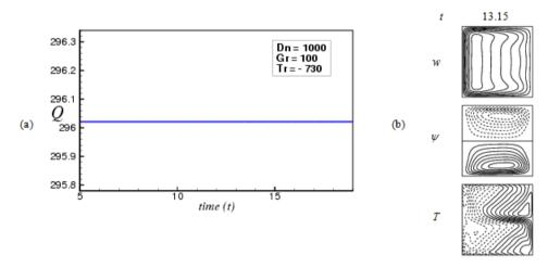
Fig. 16 Transient solution for Try = -730 (a) Q as a function of time, (b) Velocity contour (top & middle) and isotherm (bottom)
