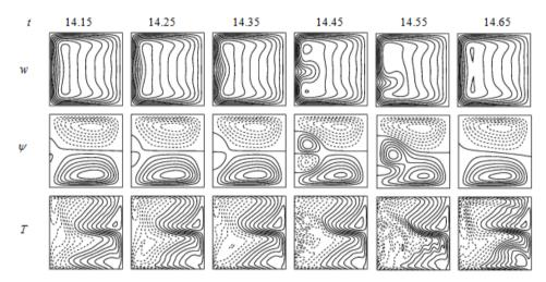
Fig. 15 Velocity contour (top & middle) and isotherm (bottom) for Try = -400
