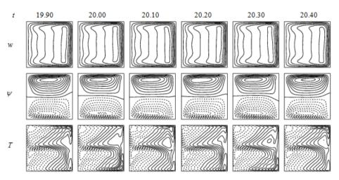
Fig. 6 Velocity contour (top & middle) and isotherm (bottom) for Tr = 900
