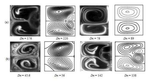
Fig. 23 Experimental (left, Yamamoto et al. [43]) vs. numerical (right, authors) results for rotating curved square duct flow; (a) Tr = 150, (b) Tr = -150
