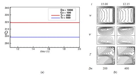
Fig. 4 Transient solution for Tr = 200 and Tr=400 (a) Q as a function of time, (b) Velocity contour (top & middle) and isotherm (bottom)
