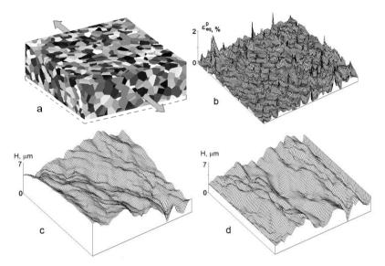
**Fig. 7** Equivalent plastic strain (b) and roughness patterns (c, d) on the free surface of the polycrystalline specimen (a) at a tensile strain of 0.4%; the boundary conditions at the lateral sides simulate the symmetry planes (b, d) or free surface (c)
