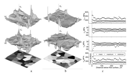
**Fig. 2** Equivalent stress and equivalent plastic strain distributions in the surface layer of polycrystal (a) and at a depth of 250 μm below the surface (b) and the maximum, minimum and mean values of stress tensor components at different depth below the free surface at 2% strain
